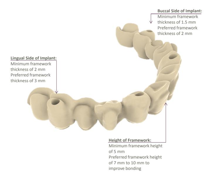
**Palatinal Plate Protection:** Required to avoid damage/de-bonding between the framework and the veneering. Where possible avoid contact between the veneer and the antagonist and ensure contact in the anterior region of the Juvora framework.
